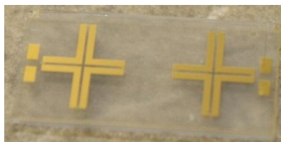
A die including 2x1 cells with 4 biasing pads; A MEMS varactor across the unit cell slot with DC bias lines.
