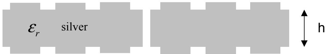
Fig. 1. Geometry of metal film layer (silver) at optical wavelengths with corrugations on both faces, and apertures connected by a small hole in the film.
