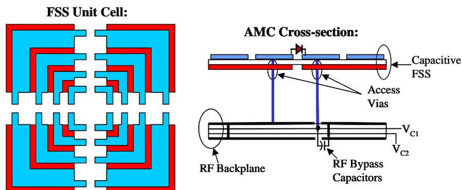
**Figure 1 - FSS unit cell & AMC cross-section showing bias via configuration**
