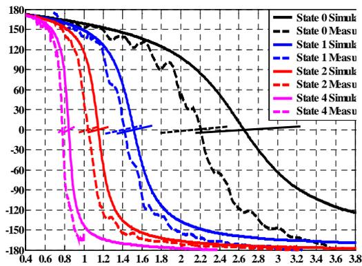
Figure 3 - AMC State 2 Geometry and Reflection Phase for Each State (Measured & Predicted). The  $\pm 90^\circ$  bands are indicated by the slant line
