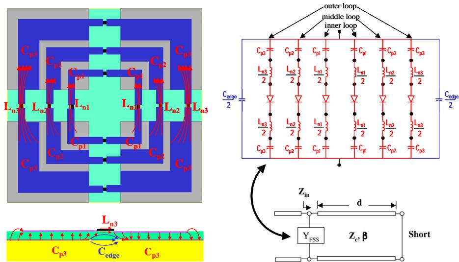
Figure 2 - Multi-loop FSS Geometry and Equivalent Circuit Model
