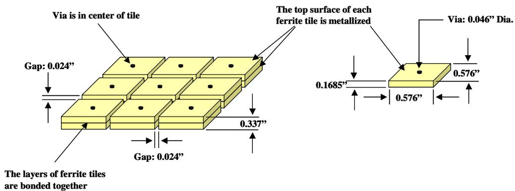
**Figure 2.** Ferrite Tile Geometry
