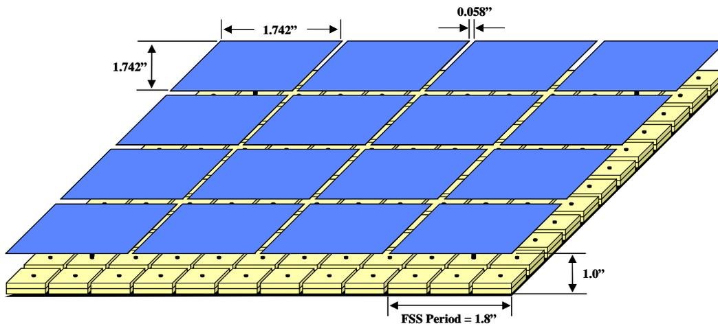
**Figure 1.** Magnetically Loaded AMC Geometry
