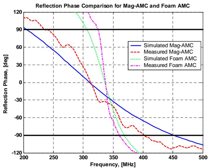
**Figure 5.** Reflection Phase Comparison for Mag-AMC and Foam Core AMC
