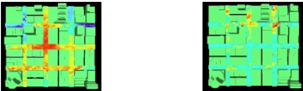
Figure 1 – AMI as a Function of Mobile Position for a Center Excited 7x7 MIMO System (A) With and (B) Without Path Loss Effects
