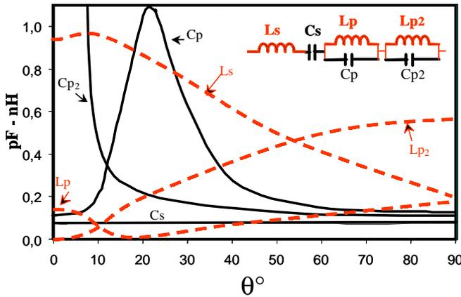
Fig. 3 Synthesized  $\theta$ -dependent L and C parameter for the TM case (the circuit for the TE case includes only one parallel-type block for the same bandwidth)
