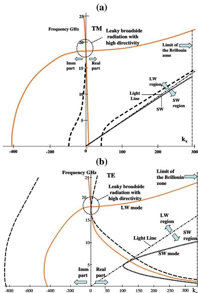
Fig. 5 Dispersion diagram for leaky and surface wave solution. (a) TM case; (b) TE case
