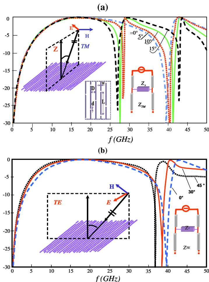
**Fig 1** Reflection coefficient of an FSS (gangbuster "type 2"  $L = 10$  mm,  $D = 2.51$  mm,  $d = 0.571$  mm,  $w = 0.25$  mm.) versus frequency for different scan angles (a) E- plane (TM) and b) H-Plane (TE).
