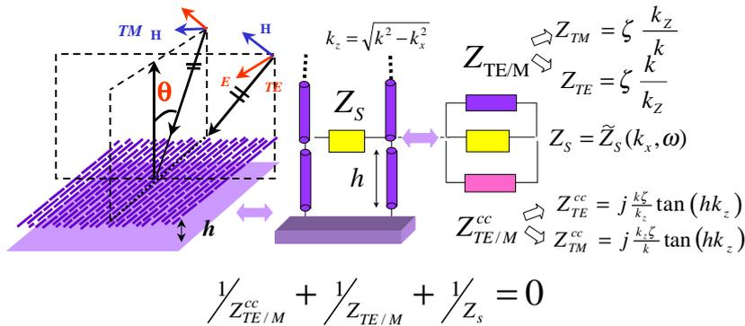
**Fig. 4** Transverse resonance equation via synthesised network for the grounded FSS
