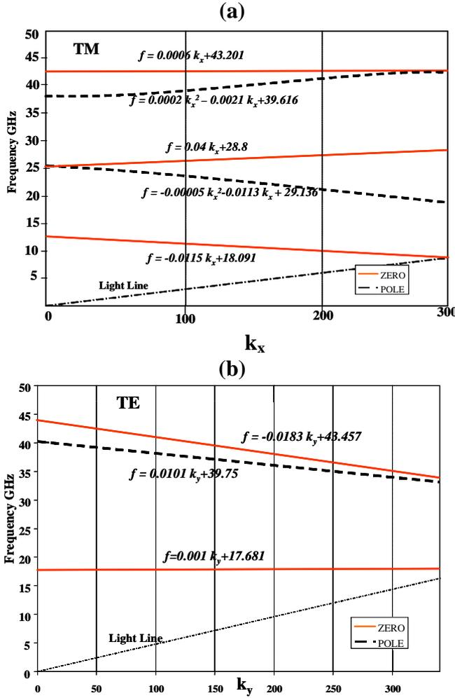
Fig. 2 Position of zeros and poles of  $Z_s$  in the  $f-k_x$  plane (TM case figure (a)) and in the  $f-k_y$  plane (TE case figure (b)).
