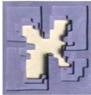
Figure 2. (Left) Fabricated substrate after filtering and modifications and its return loss performance comparison with initial and optimized volumetric graded substrate (right).
