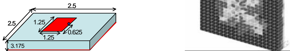
Figure 1. (Left) Schematic of patch antenna on initial homogeneous substrate (dimensions are in cm) and optimized volumetric graded substrate (right)
